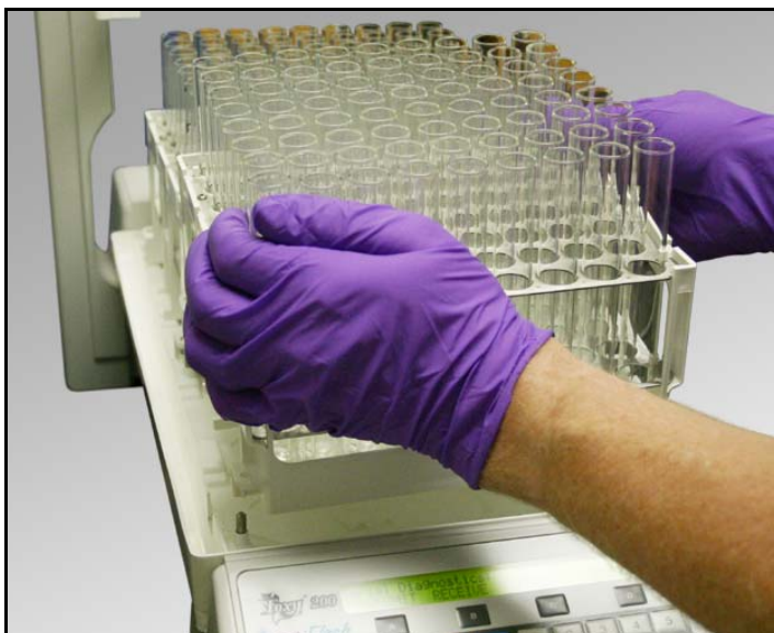
Figure 8-1 Loading the racks
