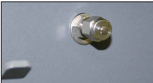
Figure 8-4 Plug sealing the Solid Sample Cartridge bulkhead fitting
