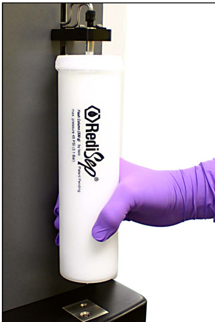
Figure 8-3 Loading a 330g RediSep Column
