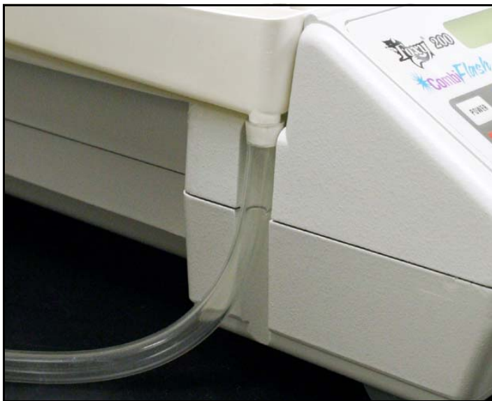
Figure 2-1 Foxy 200 Drain Tubing
