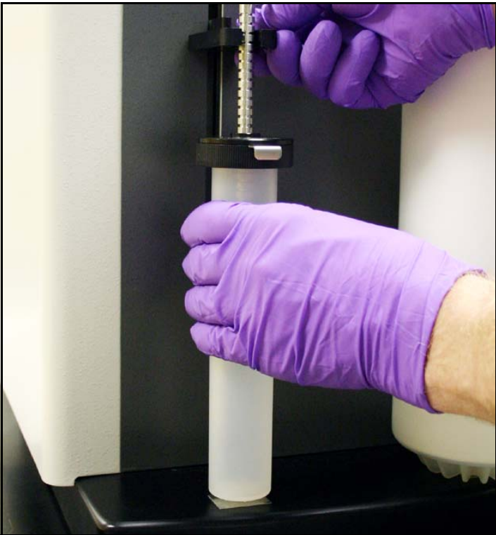
Figure 8-10 Installing the solid sample cartridge
