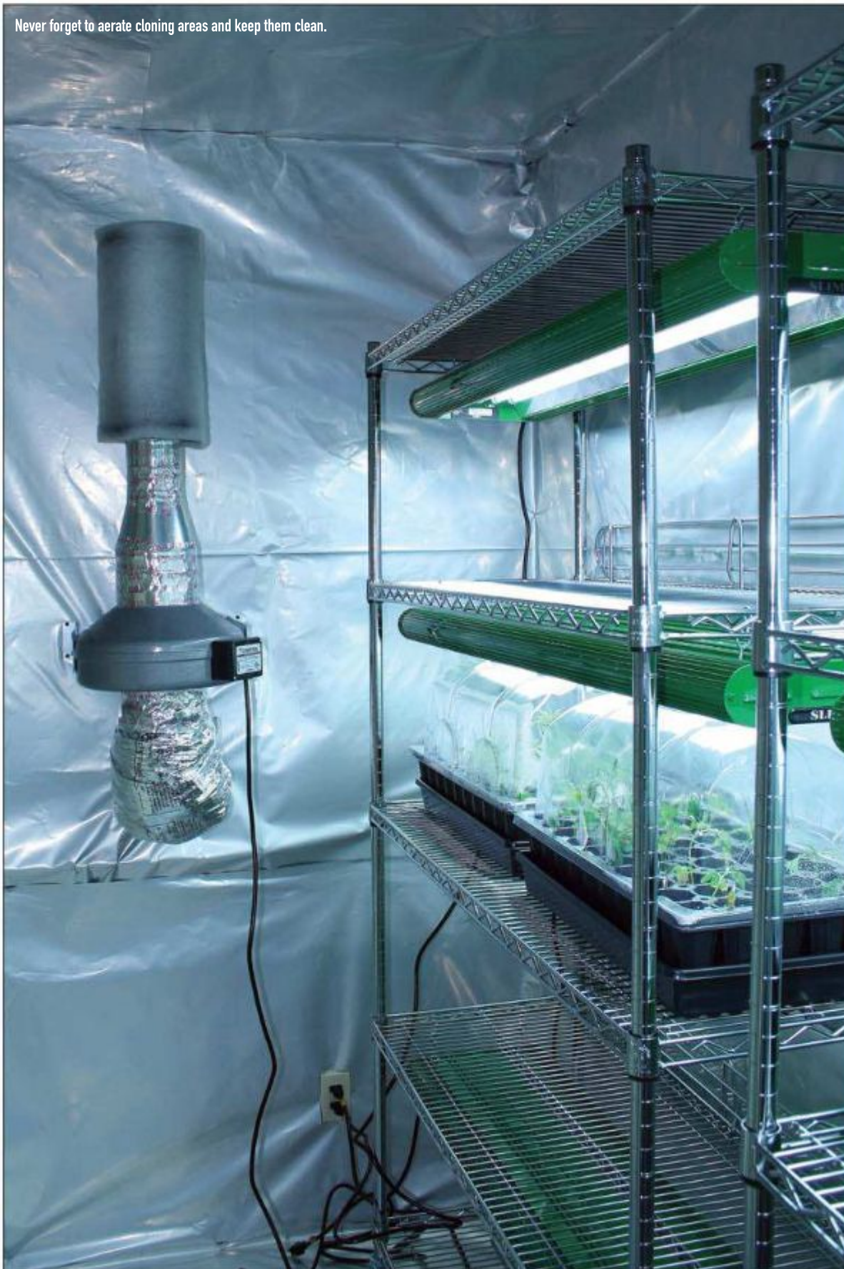
This ozone generator cleans odors as air travels through exhaust tubing.
