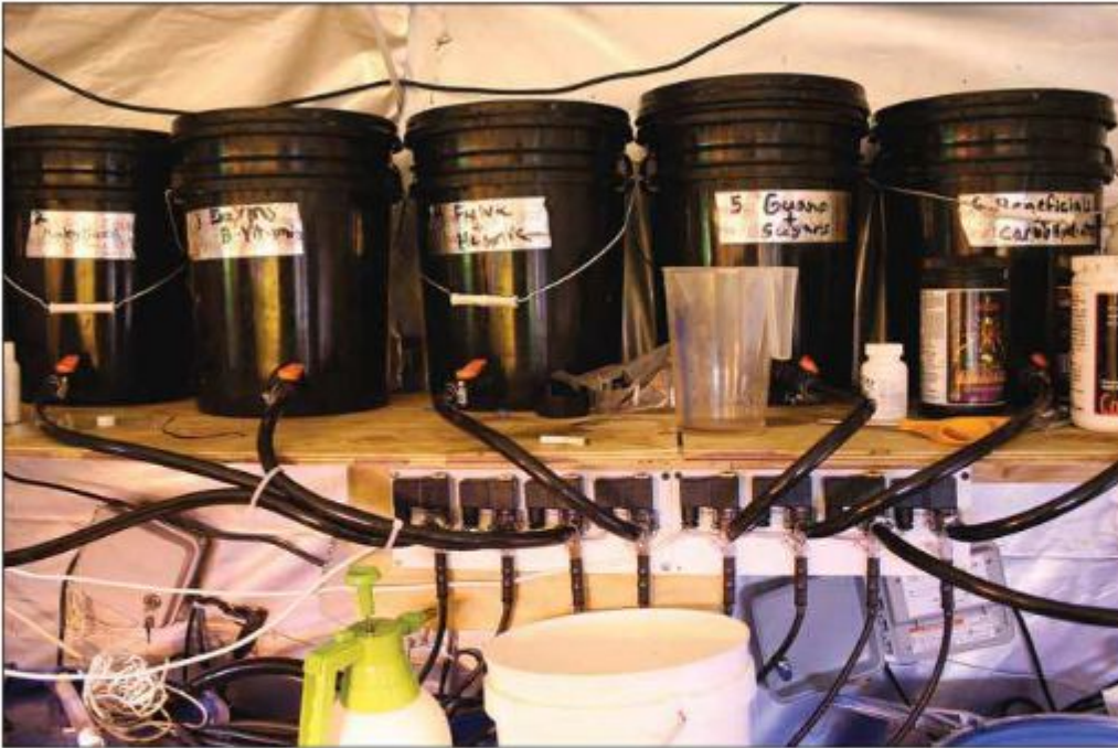
Buckets hold precisely measured nutrients ready to be automatically added to the reservoir.
