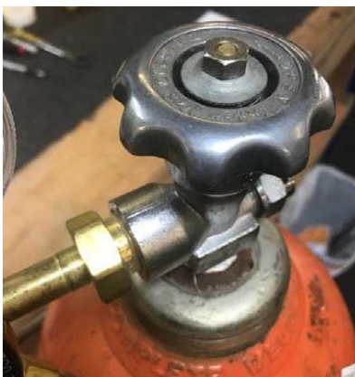
Figure 7-6: Regulator and Nitrogen Tank Connection
