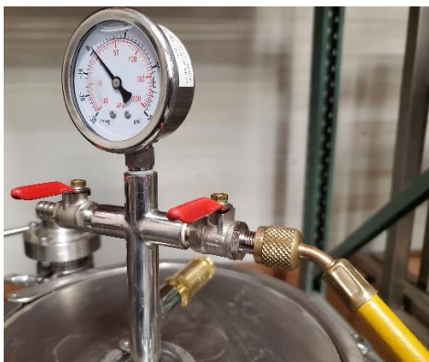
Figure 7-8: Pressure Hose to Dip Tube Manifold Connection
