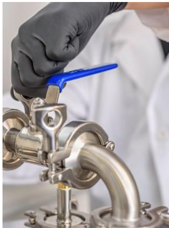
Figure 7-11: Lid Inlet Valve in Closed Position
