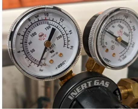
Figure 7-10: Set Regulator Pressure 15 PSI
