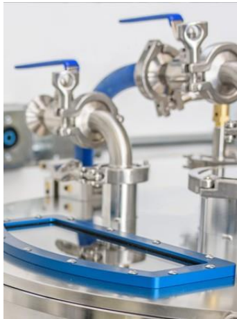
Figure 7-14: Lid Inlet and Vent Valves in Open Position
