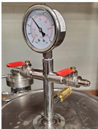
Figure 7-5: Dip Tube Manifold, Valves Closed
