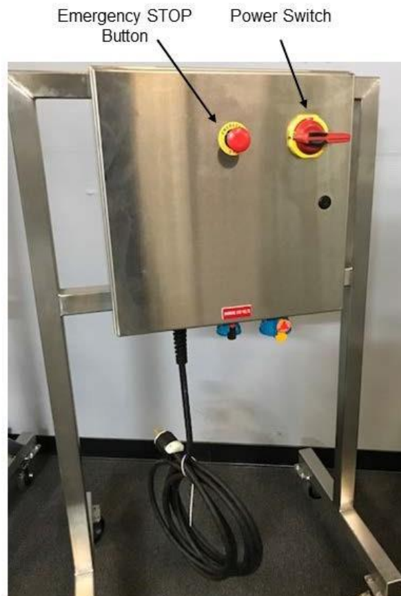
Figure 6-1: Main Control Panel
