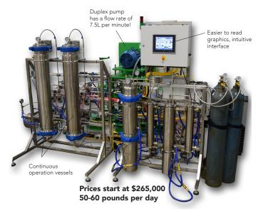
Our new system allows for continuous batch operation and is more energy efficient per pound, at just 20hp total power consumption. Our control panels have more pressure and temperature data points than any of our other systems!
