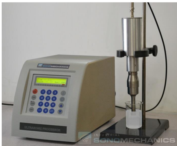
Figure 2. Laboratory-Scale Ultrasonic Liquid Processor
