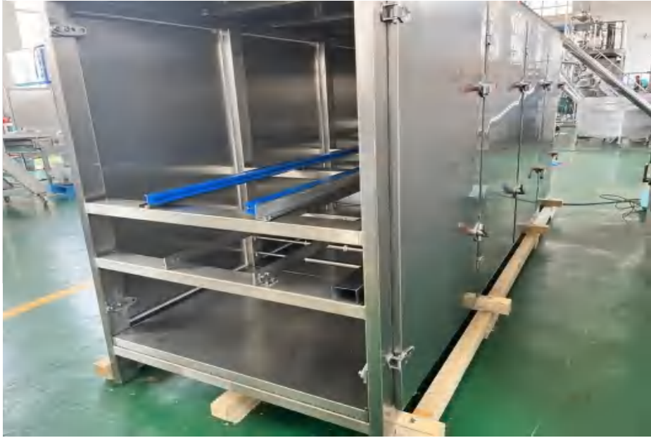
Four side cover with sandwich insulation
