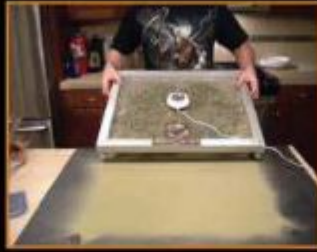
STEP 2 - LET THE LEAF DEBRIS VIBRATE FOR 5-15 MINUTES.
