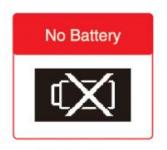
No battery install the battery Screen flashing 10s
