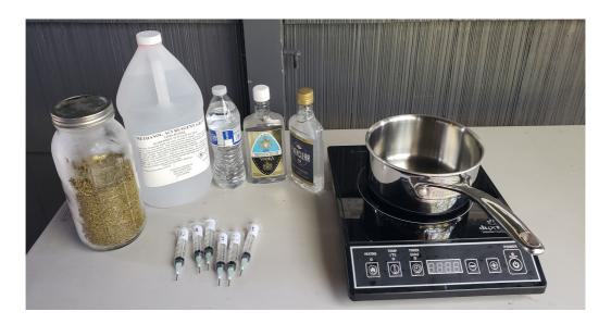
This test was performed on 6.5 ounces of dry decarboxylated plant material, ground up and placed in a 64oz mason jar. First wash was performed using Methanol ACS Reagent for 15 minutes, and a secondary rinse of the same for less than one minute. Both the priamry was and subsequent rinse was poured into a bucket, filtered through nylon mesh, then repoured into three 32oz quart mason jars. Each jar was labelled A, B, and C. Jars B and C weighed in at 23.44 oz and 23.63 oz
