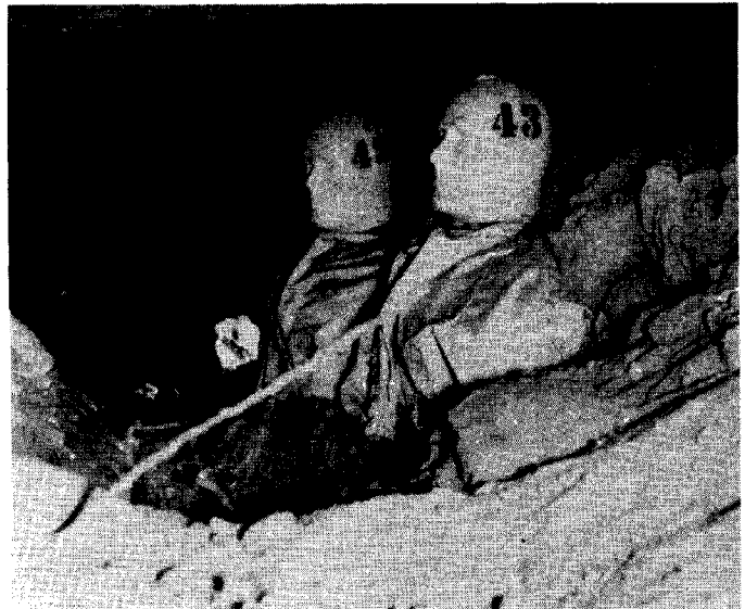
Fig. D.6. Dummies after ground shock from 1-kiloton blast effects at the 20-psi range had collapsed the rock-like walls of a hardened desert soil called caliche. The dummies' steel "bones" and "joints" prevented them from being knocked down and buried. The fallen caliche all around them kept them from being blown over by the air blast wave and 180-mph blast wind that followed.
