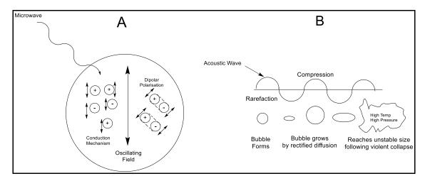
Figure 4: (A) Microwave effects on the polarizability of polar solvents, as well as local heating or superheating causing increased reaction rates. (B) Acoustic waves (sonicator) causing compression and rarefaction causing increased mechanical effects causing increased reaction kinetics.
