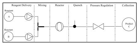
Figure 1: Six component breakdown of a basic flow system with coil reactor
