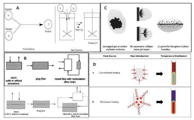
**Figure 2:** (A) comparison of the two various methods of either flow or batch chemistry. (B) The various modifications of either the top with sonication in flow or batch, bottom with microwave flow or batch (C) Microenvironments of solvated compounds caused by sonication (D) comparison of conventional heating (top) compared to microwave heating (bottom).
