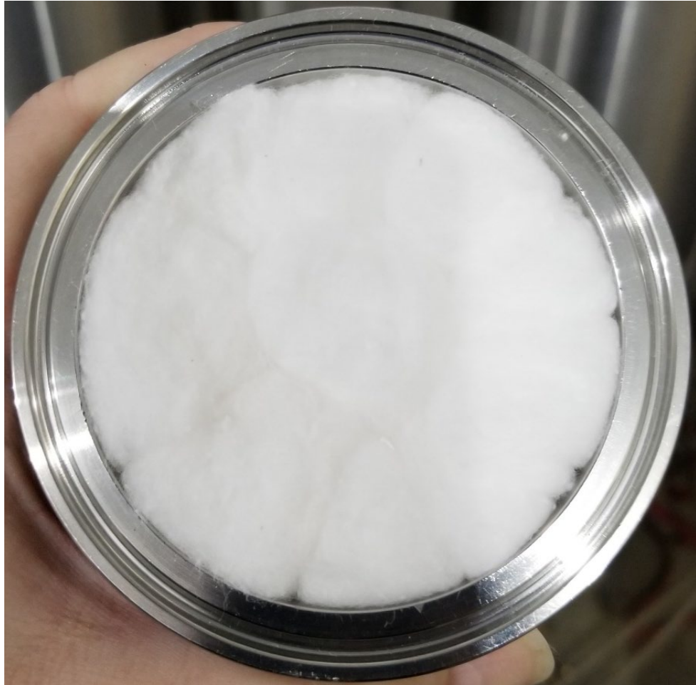
Figure 4: Cotton or Glass Fiber: Depth filter medium ...packed sufficiently tight to fit snug, but NOT overly compressed, covering all area of perforated plate and fine screen, and filling volume up (about 1 inch) to flange in Figure 3.
