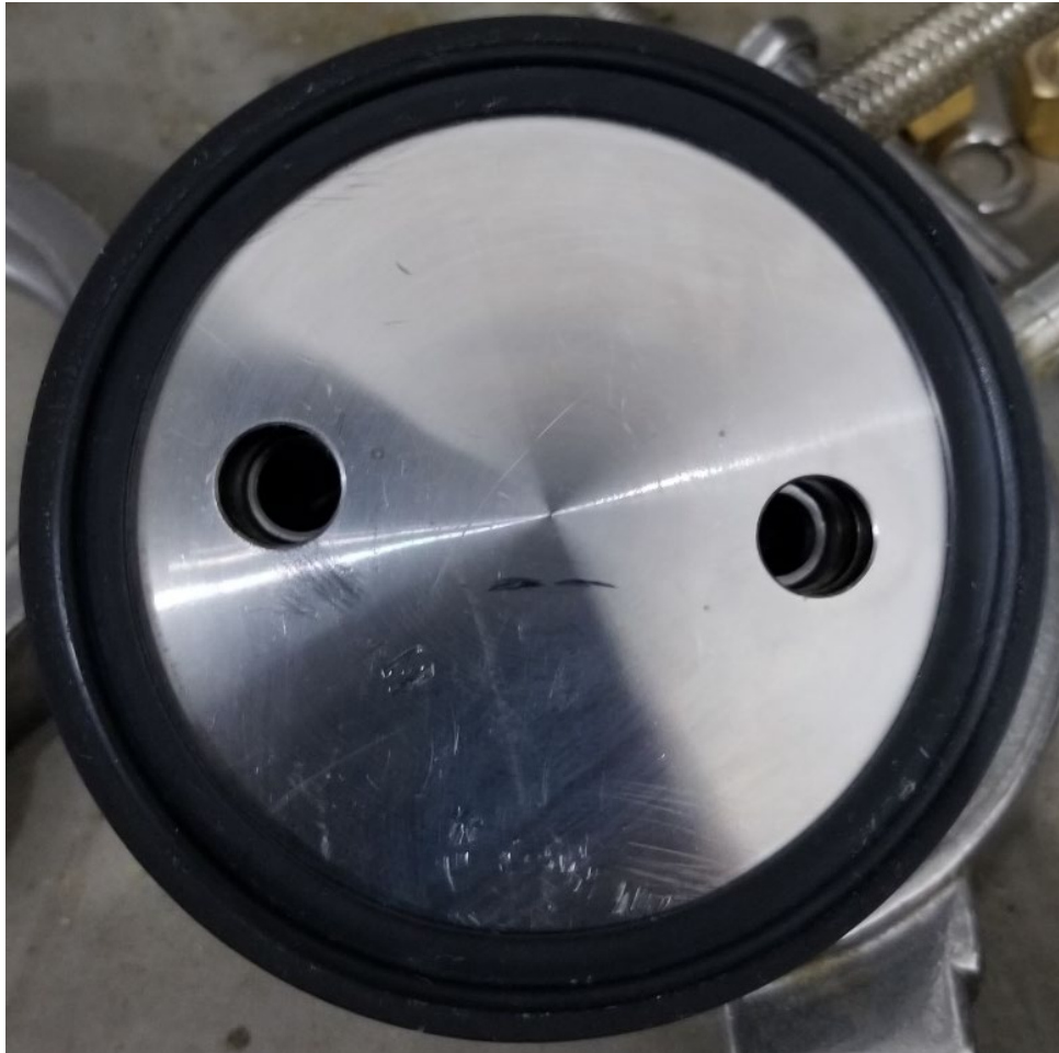
Figure 1: Sanitary Cap & Gasket: Filtrate fluid outlet ...will be attached to bottom of perforated plate segment (Figure 2) Note: This is just an example, using a flat cap with two outlet ports.
