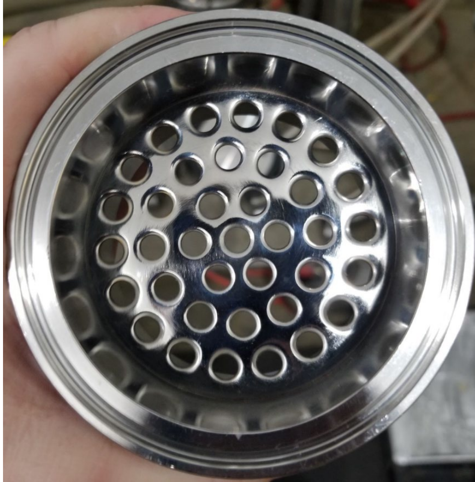
Figure 2: Top of Perforated Plate Sanitary Segment: Base support ...of depth filter fiber medium
