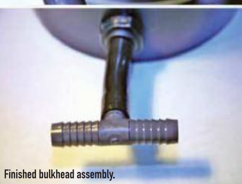
Cut 3/4" vinyl for T assembly and connection.
