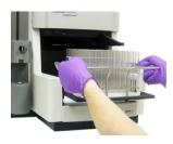
• Insert the carrier into the guides. Select the guide that places the top of the tube as high as possible under the drop former without contacting it.
