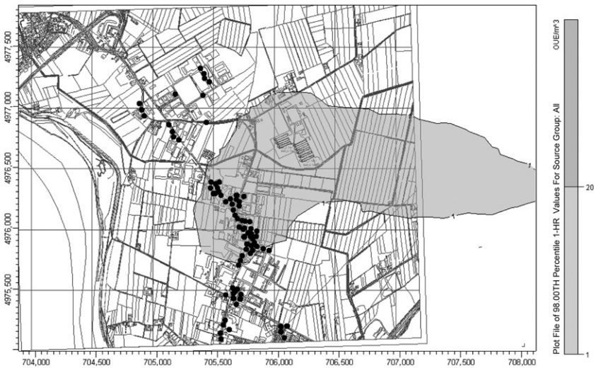
FIGURE 8 Results are reported from modeling of odor dispersions using a non-steady-state Lagrangian model (Calpuff) from an animal odor source. Dots indicate residents' complaints. The 98th percentile is reported, with isopleths reporting odor concentration in terms of OU_E/m^3 .
