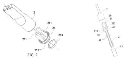
The present invention has a mouthpiece plug-in lock structure, capable of rapidly sealing and locking the open tank by means of the mouthpiece, and has advantages of being convenient and easy to mount and having a simple structure.
