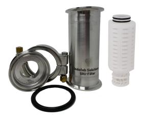
The ulti filter is a versatile tool used for micron filtration. It consists of a three inch diameter filter body and a lower sealing plate. Inside the filter housing is a replaceable filter element. The 100% polypropylene construction and viton o rings ensure wide solvent compatibility. Filter elements are available in 8 different pore sizes, making them compatible with a wide variety of tasks.
