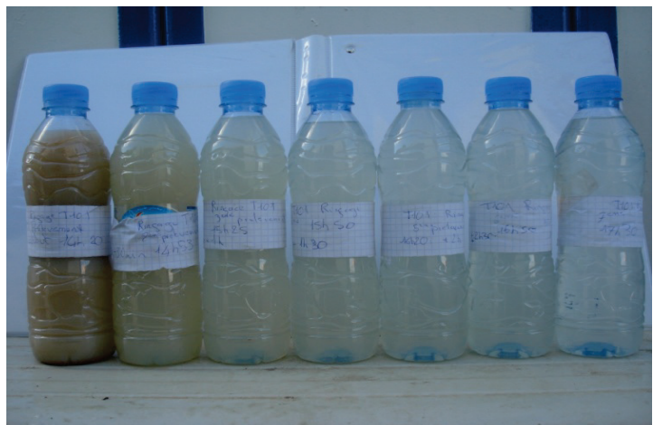
Figure 15: amine solvent obtained during the depollution operation
