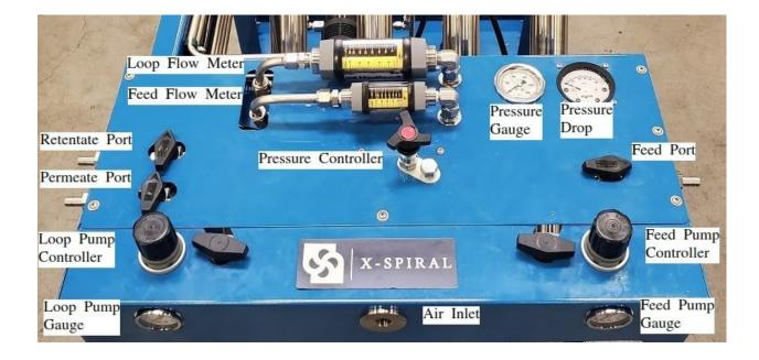
Air Inlet: Connects to the air compressor via ½" air line.
