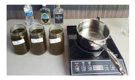
The distilling setup is a Duxtop 9100mc hotplate and a 2 quart stainless steel pot. The Duxtop hotplate was choosen for it heating control of 100 watt increments starting at 200 watts up to 1800 watts.
