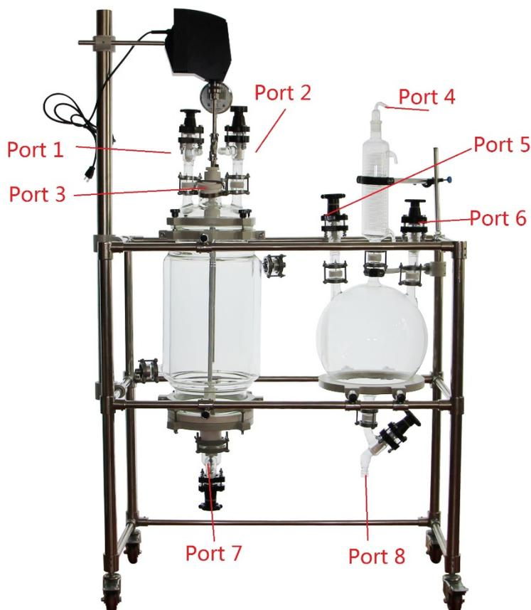
Port 1: Connect it with PTFE tube, can be used to pump in your solvent, remain close during operation
