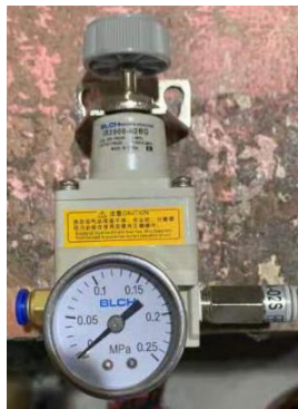
Pressure reducing valve (0.01~0.02MPa)
