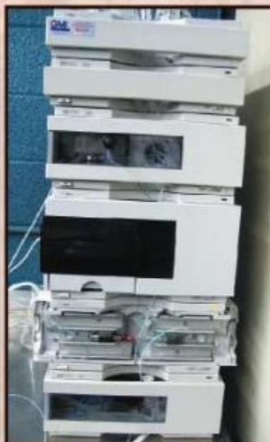
High-performance liquid chromatograph.
