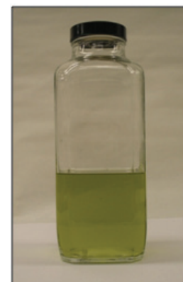
Figure 4b: Effluent from 40 Micron Polypropylene 6.2 ppm suspended solids
