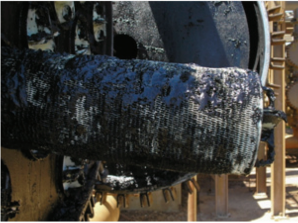
Figures 2a & 2b: Examples of "shoe polish" Contamination
