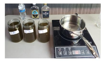
The distilling setup is a Duxtop 9100mc hotplate and a 2 quart stainless steel pot. The Duxtop hotplate was choosen for it heating control of 100 watt increments starting at 200 watts up to 1800 watts.
