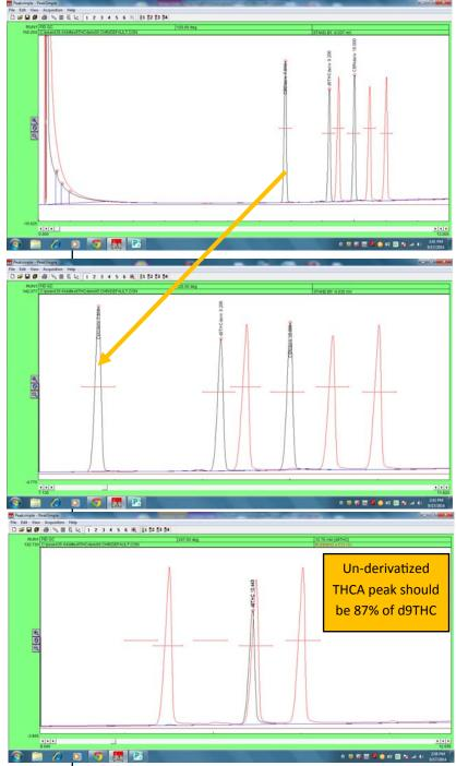
Here is the chromatogram of un-derivatized THCA (Restek# 34093) in black. Notice that the peak comes out at the same time as the d9THC. The un-derivatized THCA decarboxylates in the GC and becomes d9THC, so it makes sense that it elutes at the same time as d9THC. The size of the un-derivatized THCA peak should be 87% of the d9THC peak if the THCA standard completely de-carboxylates in the GC injector and both the 34014 and 34093 standard each contain 1000ng/ul as stated on the label.
