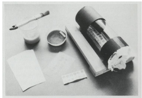
Fig. 2. Trichogramma rearing, glass cylinder, host eggs ( Sitotroga cerealella ), stripes of paper, glue brush and plastic frame
