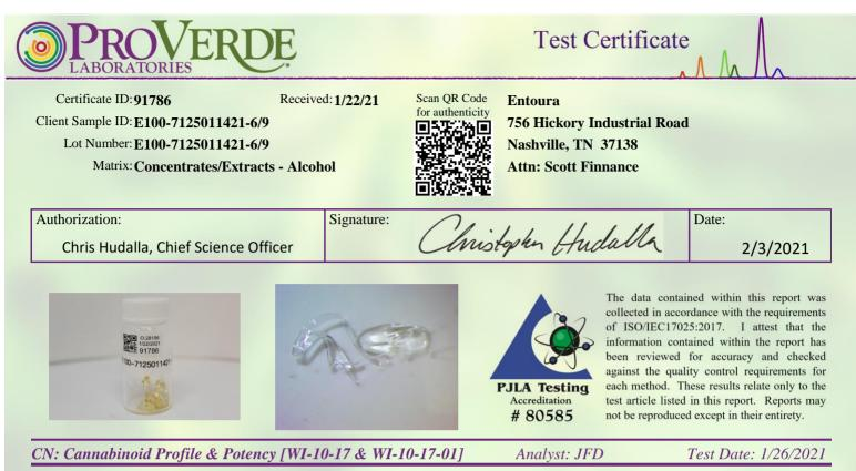
The client sample was analyzed for plant-based cannabinoids by Liquid Chromatography (LC). The collected data was compared to data collected for certified reference standards at known concentrations. In addition to compounds reported here, multiple cannabinoid isomers or byproducts, which do not occur naturally, were observed in this sample and cannot be identified. No toxicity data is available for these unknown compounds, and as such would not be recommended for human consumption.
