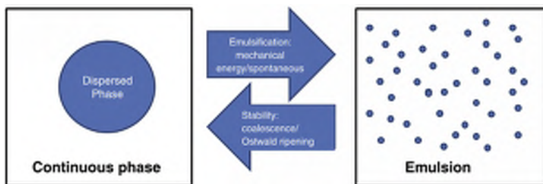
Figure 20.1. Schematics of emulsification by mechanical energy or spontaneous method.
