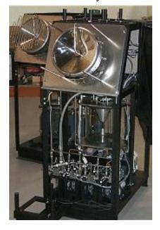
distills material at the most efficient rate per area of distilling surface. Thus, there is minimal time for decomposition.
