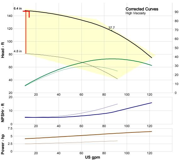
Max temp for foot-mount MAXP pump w/SmCo Magnets is 550F. Centerline mount available to 800F. Max HP/100 rpm for magnet frame indicated in magnet size is F&S=1.22; M=2.55; & L=6.33
