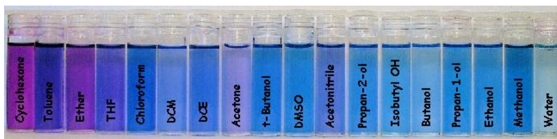
Figure 3.9 Change in absorbance of phenol blue shown for solvents ranging from nonpolar cyclohexane, to polar water
