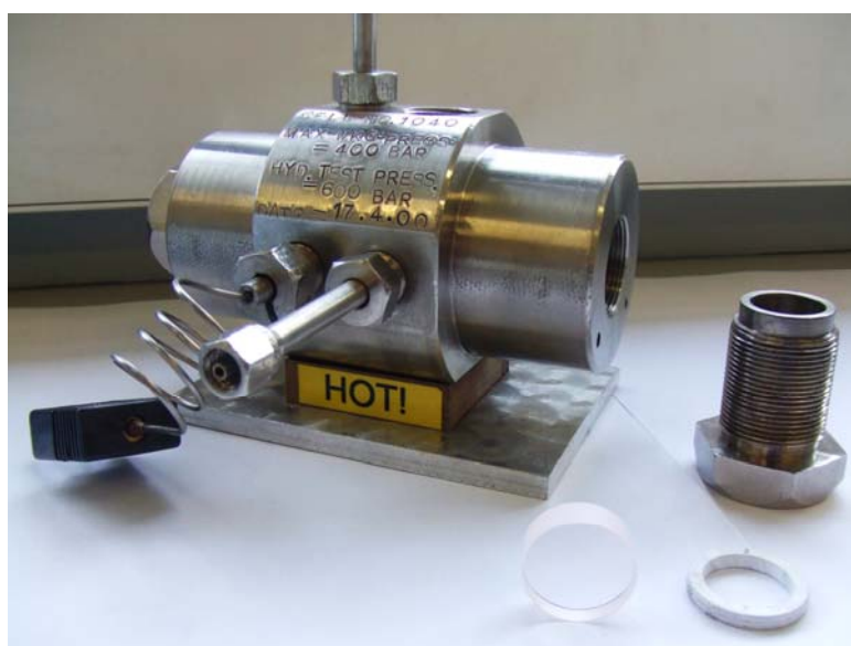
Figure 2.9 High pressure view cell used for visual observations
