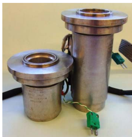
Figure 2.8 High pressure vessels used for reaction chemistry, with 50 mL, and 100 mL volume capabilities. Cells are constructed of 316 Stainless Steel and rated to 300 bar
