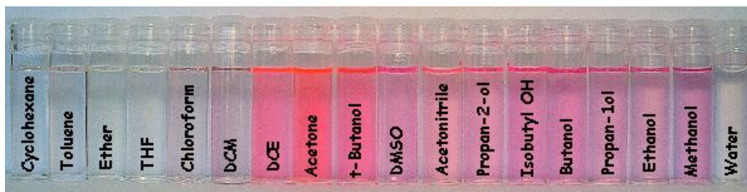
Figure 3.12 Nile Red in a range of solvents with increasing polarity from left to right
